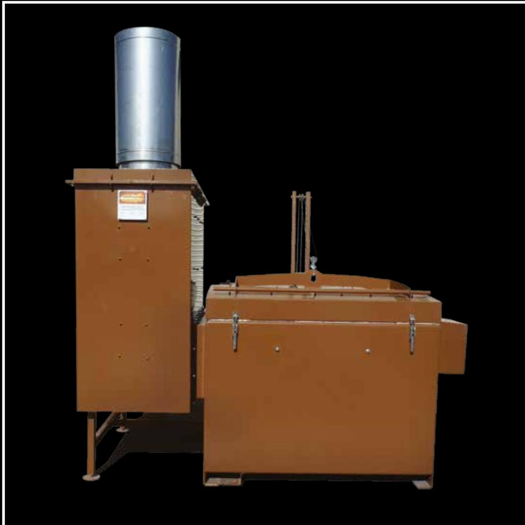
**NB50-50** 0.5 cubic metre capacity suitable for small sheep, free range poultry units, pet cremation.
